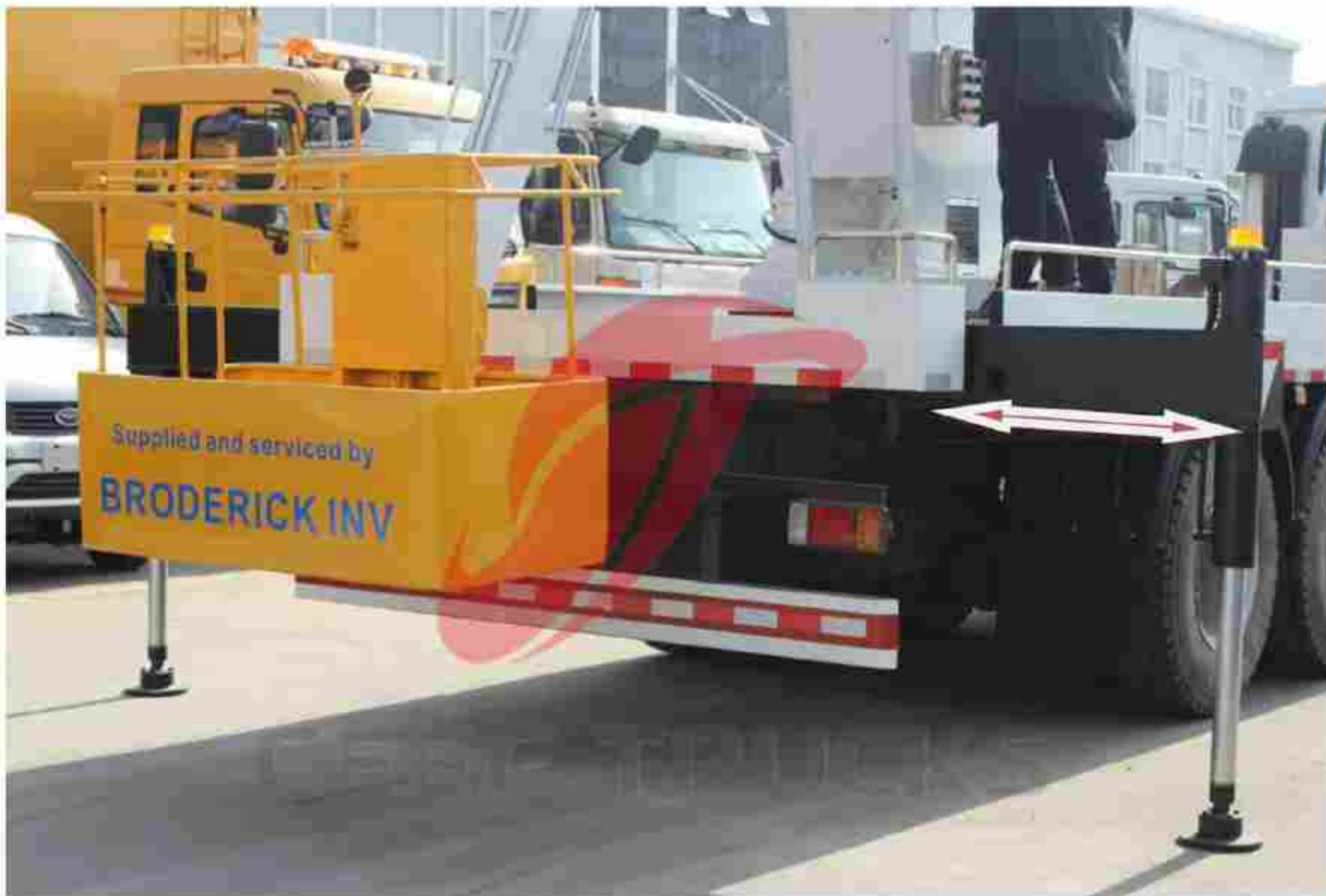
The Arrow in the picture show the Hydraulic legs horizontal direction move
